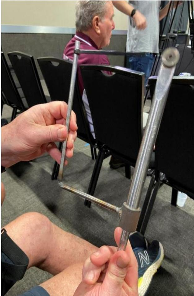
To the left is one of Neil's deep hole boring tools and how he uses a cable tie to work out the wall thickness
