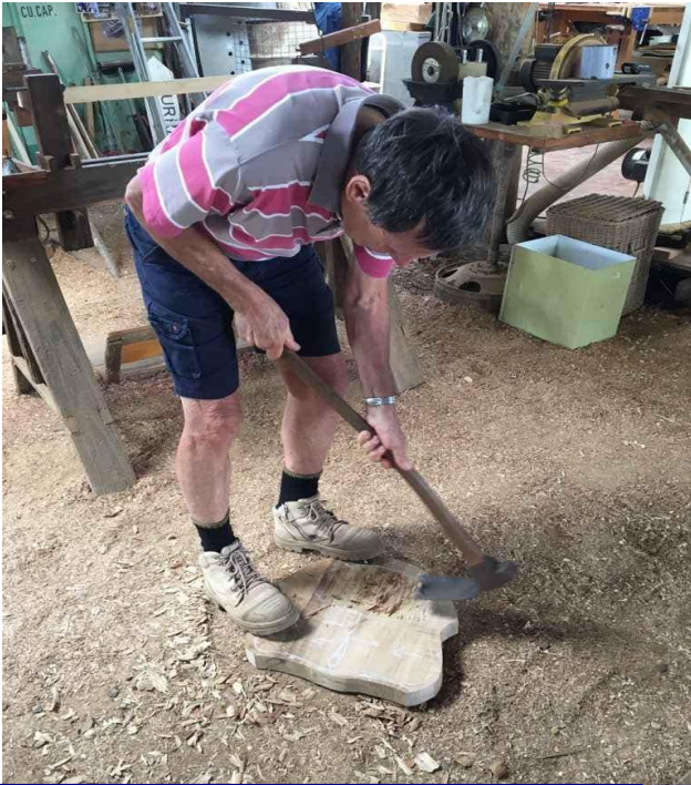
Starting to shape the seat with an adze
