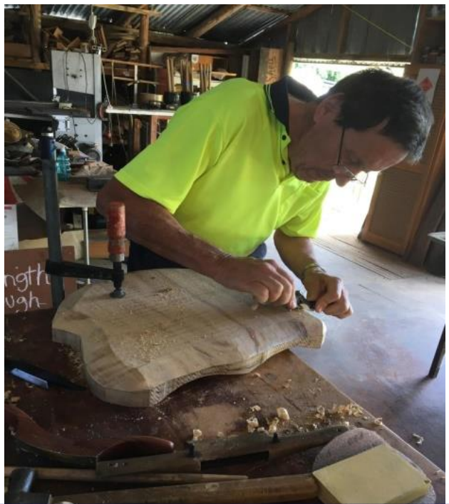
Shaping the edge of the seat with a spoke shave
